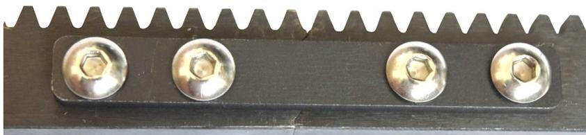
It is recommended that oil is applied to the racks and clamp pieces every 4 months or so - this is not needed for mechanical lubrication but will help defend against corrosion (particularly in higher humidity environments). Wiping along the racks with a well-oiled rag should be sufficient for this purpose.
